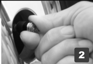
Twist the cap on to the valve stem
